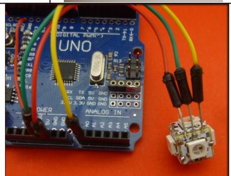
Run a test programs. If not good, check the welds with a magnifying glass by lighting at different angles with a flashlight..
